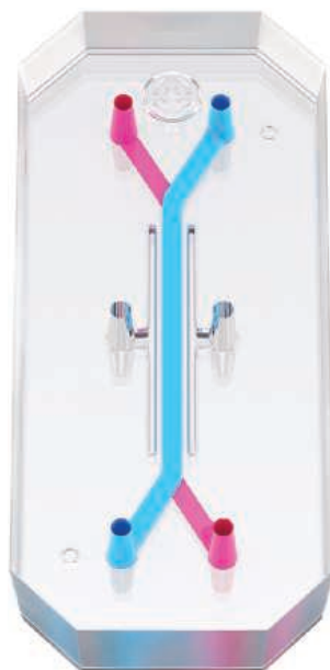
A liver chip made by Emulate contains cells and fluids found in the human liver.
